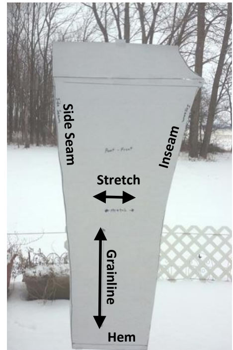
Pant leg pattern—does not extend up to waist or over pocket and zipper area.
